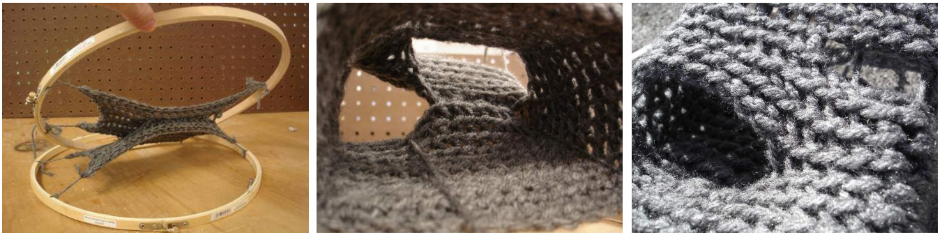
Figure 35-37: Analog experiments in creating new forms and spaces using a jig or formwork to engage the textile and enable the manipulation of the pliant model. In setting these rules, the textile model can be opened, closed, anchored, or stretched. The possibilities are only bound by the designer.
