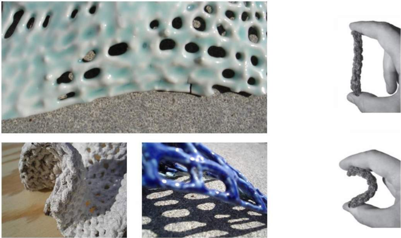
Figures 25-27: Experiments in hardening of crochet textiles using porcelain slip and plaster of paris. Figures 28 and 29: Lacquer agent used results in embedded memory of crochet threads.
